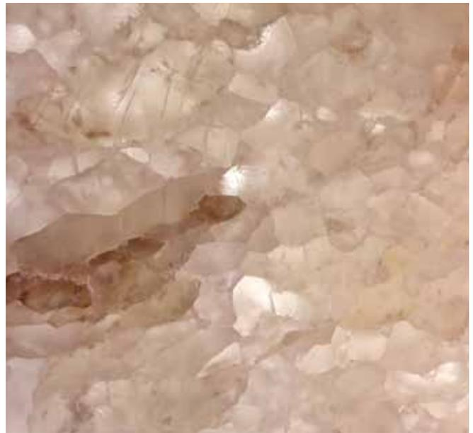
Rock salt is a sedimentary rock – it has a crystalline structure and unique properties for energy storage
